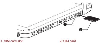
(Sample Illustration) Inserting a SIM card
